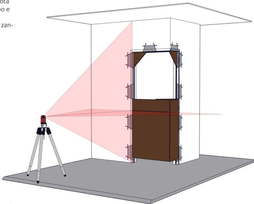
**3** Proceed in positioning the aluminum frame with the help of the laser level, to get sure that the level of the finished floor is respected, so as the squaring with the adjacent wall and the perpendicularity with it. Fix the little steel plates with cement mortar.
