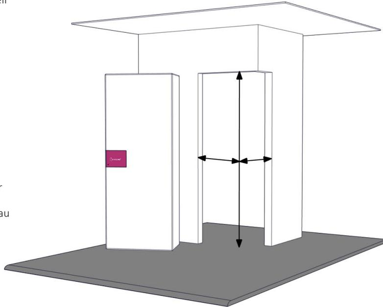
**1** Get sure that you are mounting the door which corresponds to the right opening in the wall. To ensure this, you can refer to the identification number which is printed on the package.
