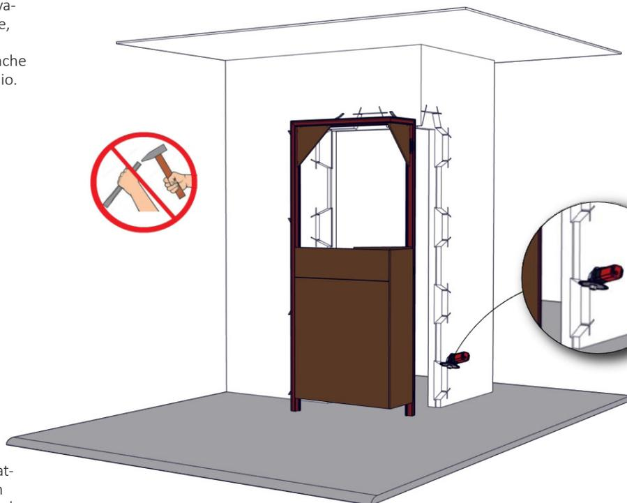
**2** Proceed with the preparation of the wall with the help of a flexible disk. Make some holes to lodge the little steel plates which are fixed on the frame. Before doing that, you have to open the little steel plates.
