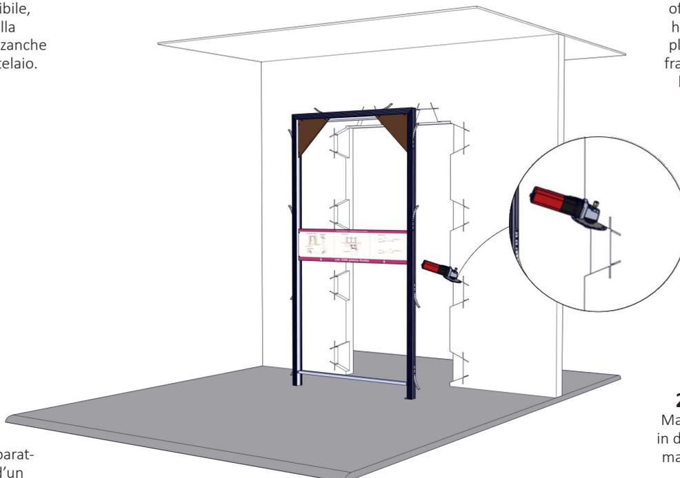
**2** Proceed with the preparation of the wall with the help of a flexible disk. Make some holes to lodge the little steel plates which are fixed on the frame. Before doing that, you have to open the little steel plates.
