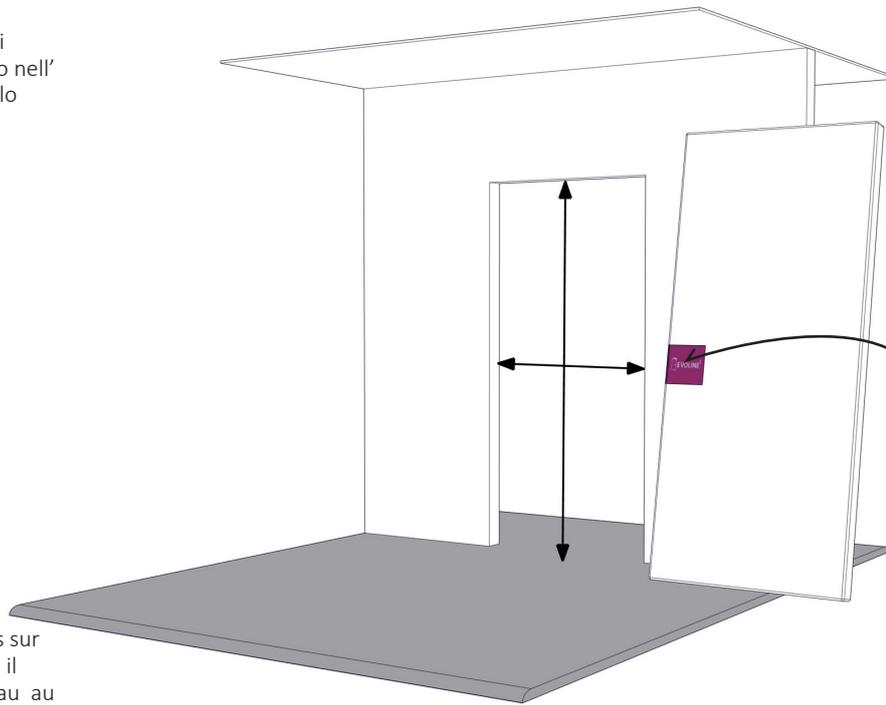
**1** Get sure that you are mounting the door which corresponds to the right opening in the wall. To ensure this, you can refer to the identification number which is printed on the package.
