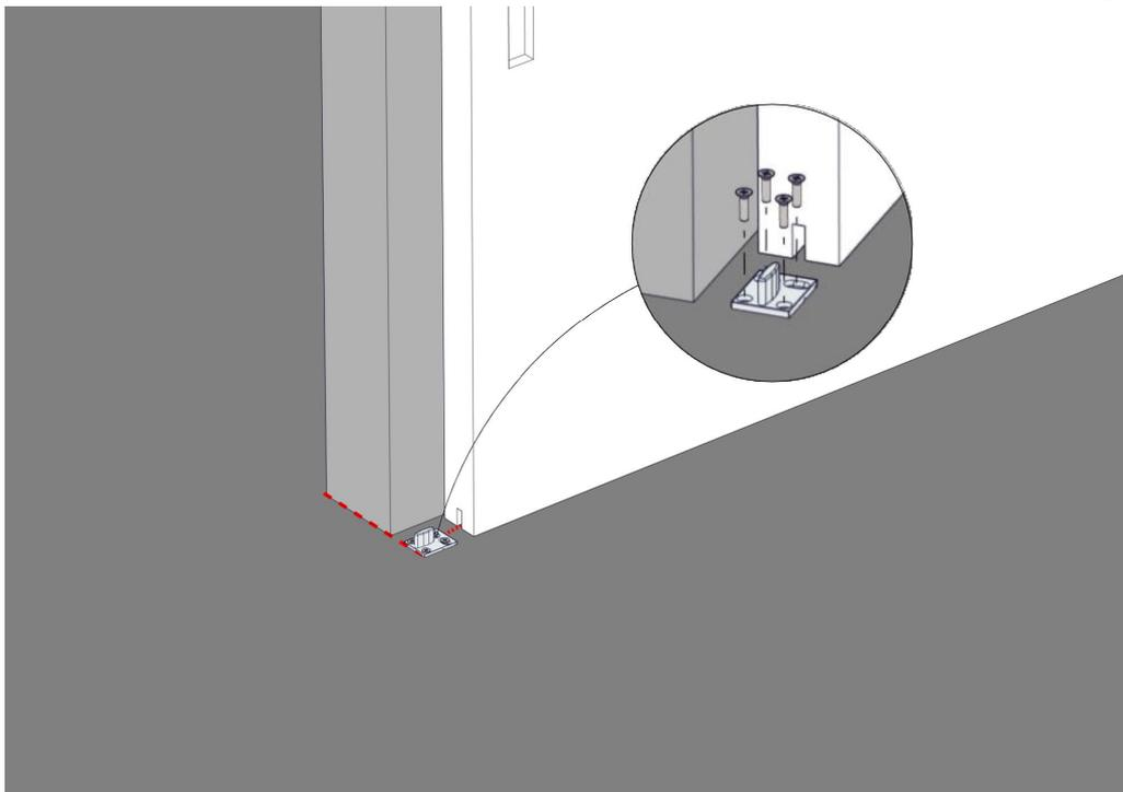
**4** Place and fix the rail on the ground in axis with the door panel
