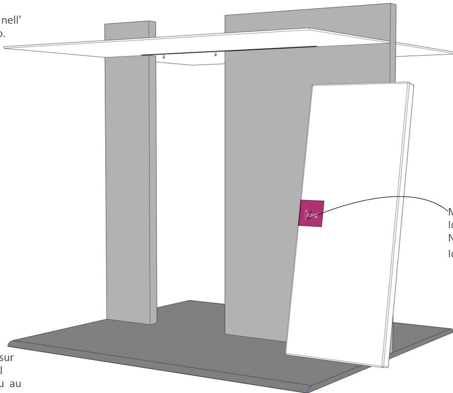
**1** Get sure that you are mounting the panel which corresponds to the right opening in the wall. To ensure this, you can refer to the identification number which is printed on the package.
