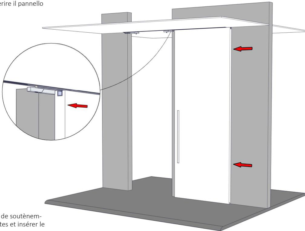
**3** Screw the support kit to the wheels and insert the door panel
