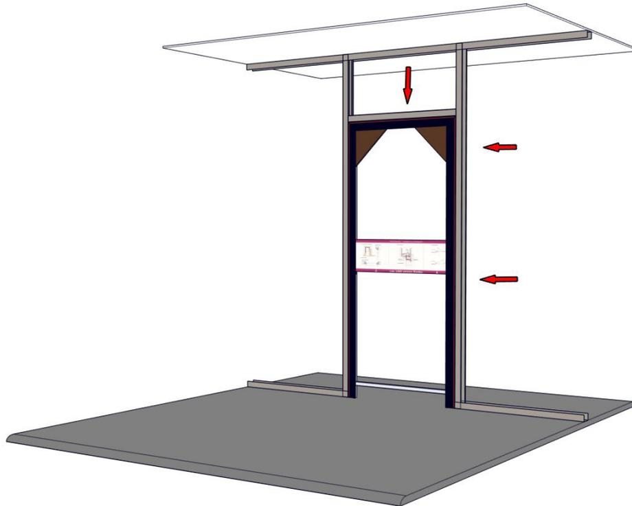
**4** Complete the structure and the fixing of the frame in bringing the parts together
