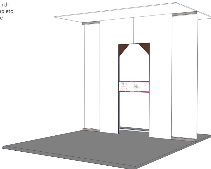
**6** The removeable spacers should be removed from the doorframe only after the plasterboard sheets have been definitively fixed on both sides
