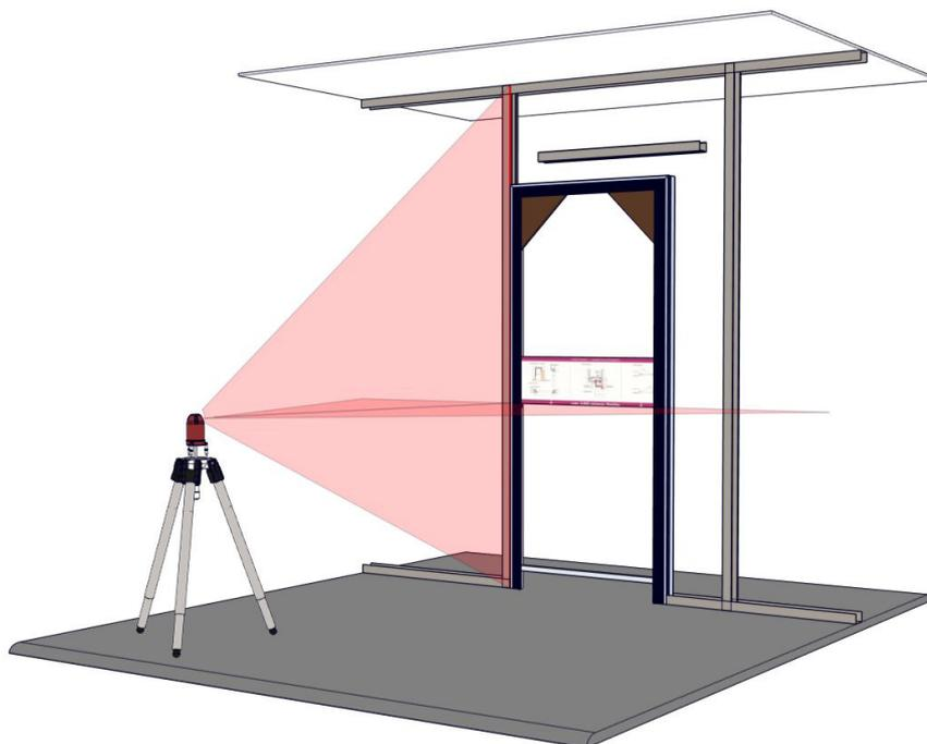
**3** Fix the frame onto the structure by following the instructions printed on the central removable spacer, to assure the right positioning of the frame
